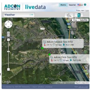
If you use an area's node ID as a URL parameter, LiveData recursively searches in the subnodes for nodes that apply to the template. If a node is visible as outlined above, the node is displayed on the map.
